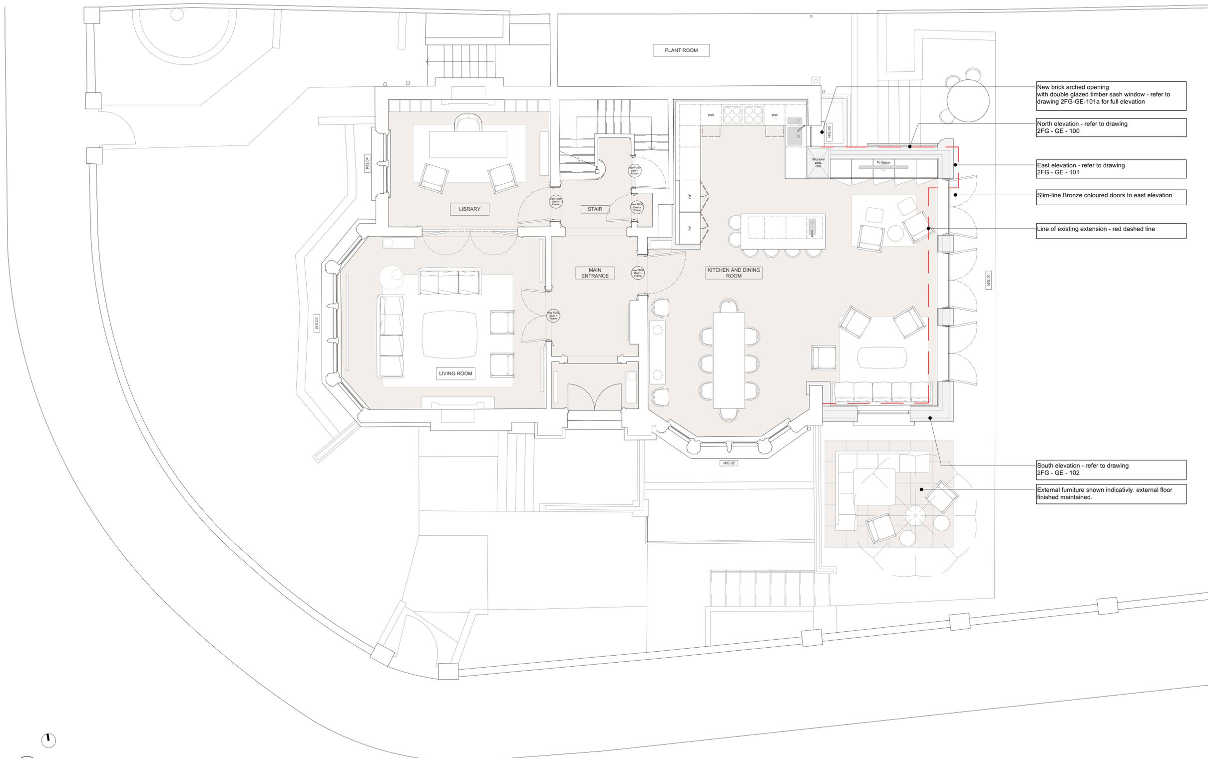
New brick arched opening with double glazed timber sash window - refer to drawing 2FG-GE-101a for full elevation
