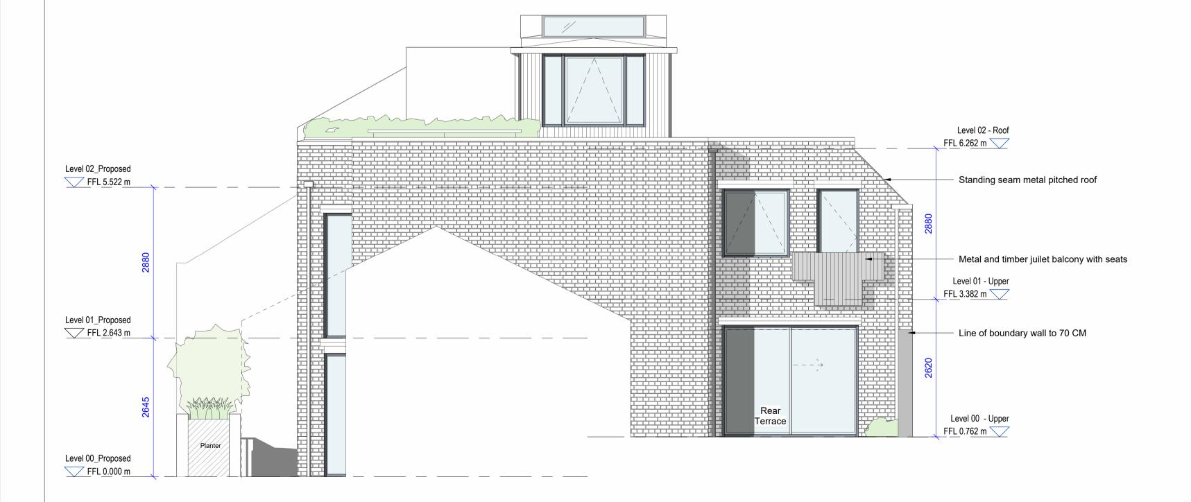
3 Side (South) Elevation\_Proposed
